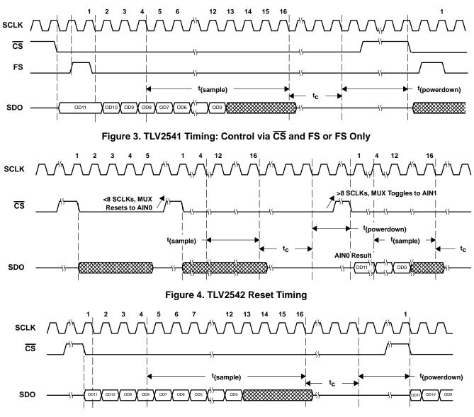
Figure 5. TLV2542 and TLV2545 Timing
