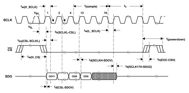
Figure 9. TLV2542 and TLV2545 Conversion Cycle Critical Timing
