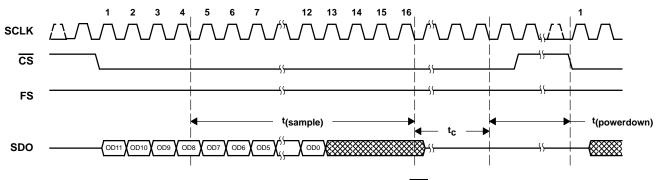
Figure 2. TLV2541 Timing: Control via  $\overline{CS}$  (FS = 1)
