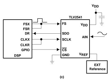
Figure 29. Typical TLV2541 Interface to a TMS320 DSP
