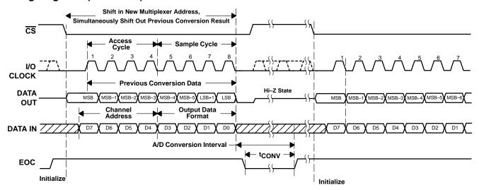
Figure 35. Timing for 8-Clock Transfer Using CS With DATA OUT Set for MSB First
