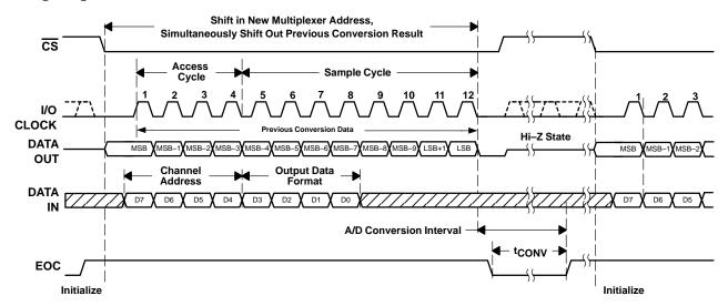
Figure 33. Timing for 12-Clock Transfer Using CS With DATA OUT Set for MSB First
