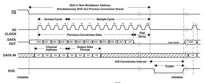
Figure 38. Timing for 16-Clock Transfer Not Using CS With DATA OUT Set for MSB First
