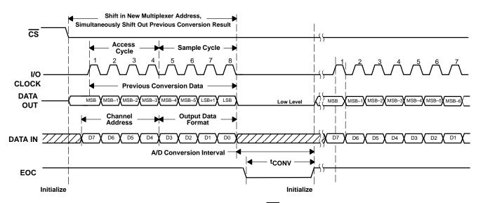
Figure 36. Timing for 8-Clock Transfer Not Using CS With DATA OUT Set for MSB First
