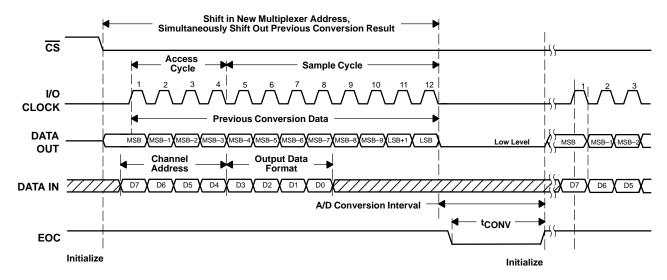
Figure 34. Timing for 12-Clock Transfer Not Using CS With DATA OUT Set for MSB First
