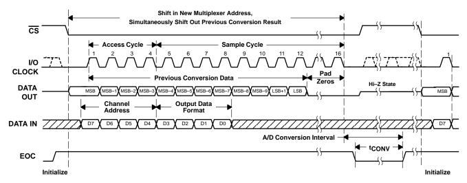
Figure 37. Timing for 16-Clock Transfer Using CS With DATA OUT Set for MSB First
