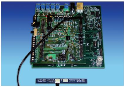
Reference Design PCB featuring TI's codec and Akustica's digital microphone array evaluation module.
