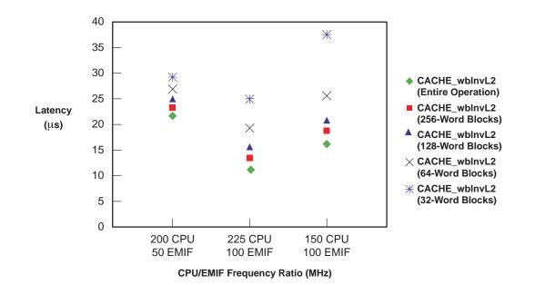
Figure 5. 1024-Word L2 Writeback-Invalidate Performance at Various Frequency Ratios With Old and New CACHE-wblnvL2()
