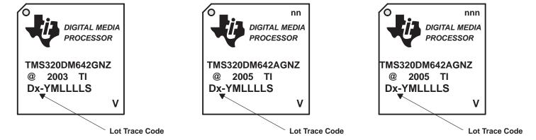
"nn" and "nnn" represent the device speed for the -500, -600 and -720 MHz devices **only** (both commercial and extended temperature).
