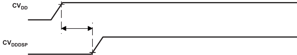
Figure 6-4. DSP Host-Boot Mode Core Supply Timings
