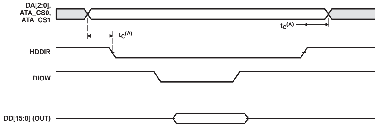
Figure 6-38. ATA/CF HDDIR Taskfile Write/Single PIO Write Timing
