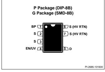
Figure 3. Pin Configuration.
