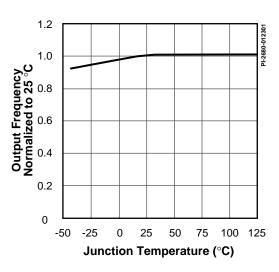
Figure 23. Frequency vs. Temperature.
