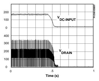
Figure 12. Normal Power-down Timing (without UV).
