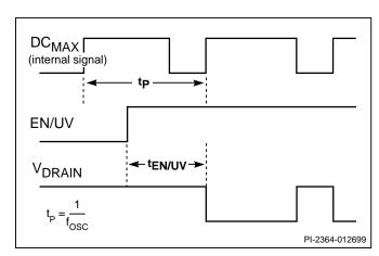
Figure 20. TinySwitch-II Output Enable Timing.
