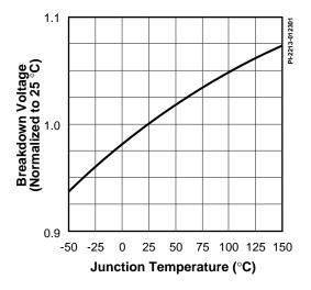
Figure 22. Breakdown vs. Temperature.
