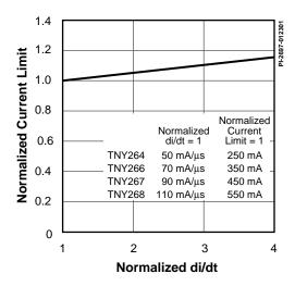
Figure 25. Current Limit vs. di/dt.
