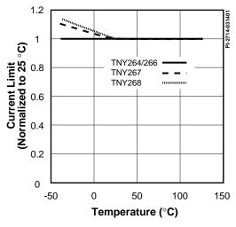
Figure 24. Current Limit vs. Temperature.
