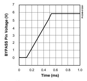
Figure 26. Bypass Pin Start-up Waveform.
