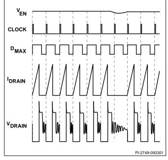
Figure 6. TinySwitch-II Operation at Near Maximum Loading.
