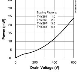
Figure 29. Drain Capacitance Power.
