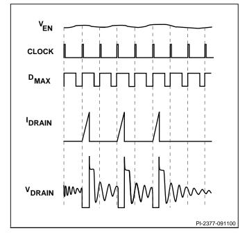
Figure 8. TinySwitch-II Operation at Medium Loading.
