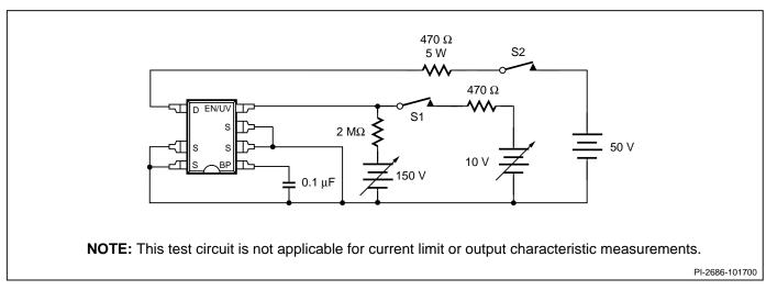
Figure 18. TinySwitch-II General Test Circuit.
