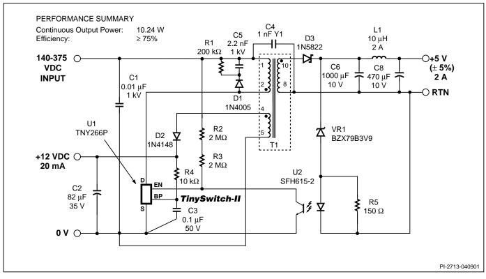
Figure 15. 10 W PC Standby Supply.
