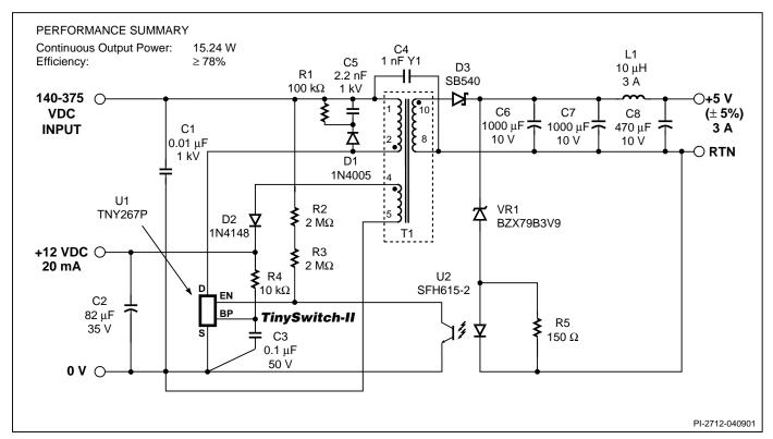
Figure 16. 15 W PC Standby Supply.
