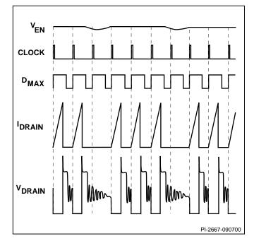
Figure 7. TinySwitch-II Operation at Moderately Heavy Loading.
