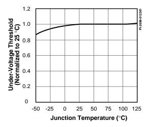
Figure 30. Undervoltage Threshold vs. Temperature.
