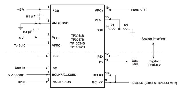
NOTE A: Transmit gain = 20 log  $\left(\frac{R1 + R2}{R2}\right)$ ,  $(R1 + R2) \ge 10 \text{ k}\Omega$
