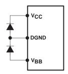
Figure 3. Latch-Up Protection Diode Connection
