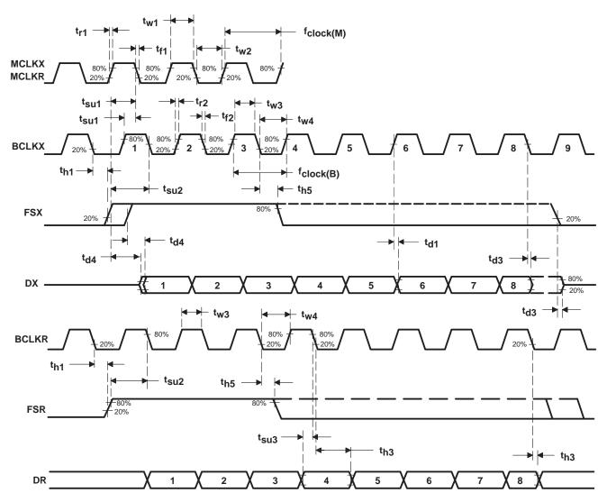
Figure 2. Long-Frame Sync Timing
