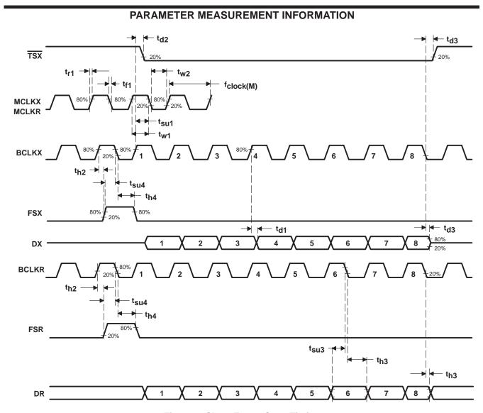
Figure 1. Short-Frame Sync Timing
