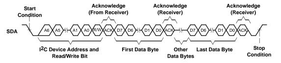
Figure 29. Multiple Byte Write Transfer
