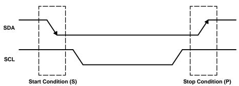
Figure 26. I<sup>2</sup>C Start and Stop Conditions
