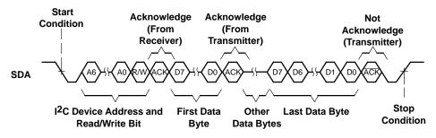
Figure 31. Multiple Byte Read Transfer
