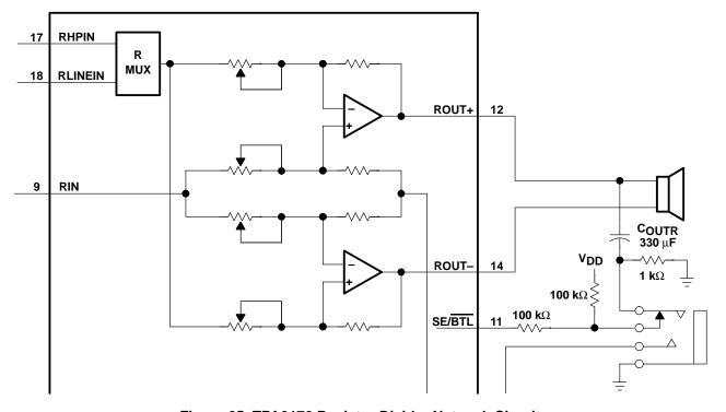
Figure 25. TPA0172 Resistor Divider Network Circuit
