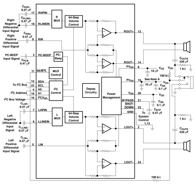
NOTE A: A 0.1-μF ceramic capacitor should be placed as close as possible to the IC. For filtering lower-frequency noise signals, a larger electrolytic capacitor of 10 μF or greater should be placed near the audio power amplifier.
