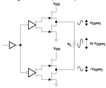
Figure 22. Bridge-Tied Load Configuration
