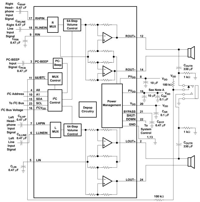
NOTE A: A  $0.1-\mu F$  ceramic capacitor should be placed as close as possible to the IC. For filtering lower-frequency noise signals, a larger electrolytic capacitor of 10  $\mu F$  or greater should be placed near the audio power amplifier.
