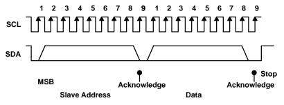
Figure 27. I<sup>2</sup>C Access Cycles
