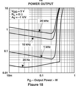
**SUPPLY RIPPLE REJECTION RATIO**
