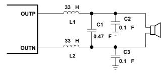
Figure 25. Typical LC Output Filter, Cutoff Frequency of 27 kHz, Speaker Impedance = 8  $\Omega$
