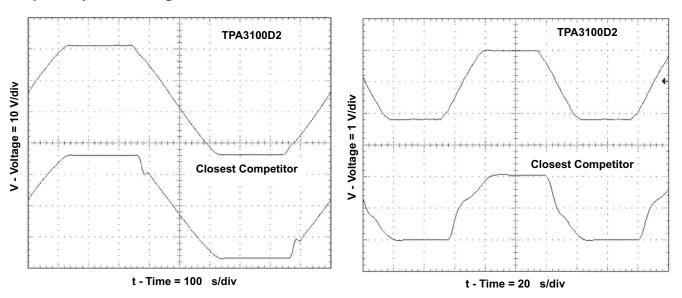
Figure 29. 1-kHz Sine Output at 10% THD+N
