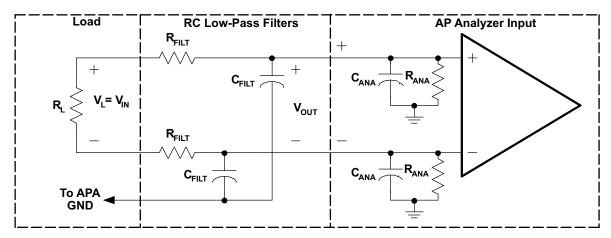
Figure 34. Measurement Low-Pass Filter Derivation Circuit-Class-D APAs
