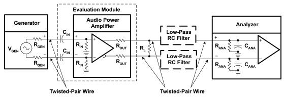
Figure 33. Differential Input, BTL Output Measurement Circuit
