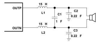
Figure 26. Typical LC Output Filter, Cutoff Frequency of 27 kHz, Speaker Impedance = 4  $\Omega$
