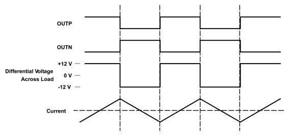
Figure 23. Traditional Class-D Modulation Scheme's Output Voltage and Current Waveforms into an Inductive Load With No Input
