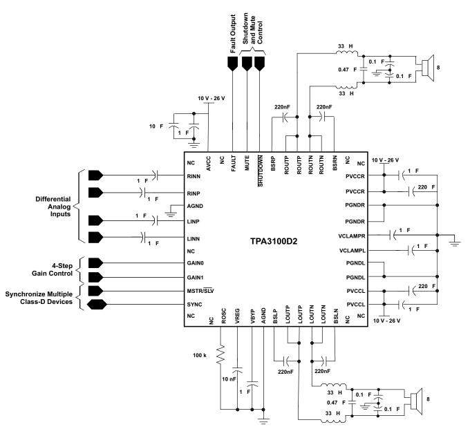
Figure 21. Stereo Class-D With Differential Inputs (QFN)
