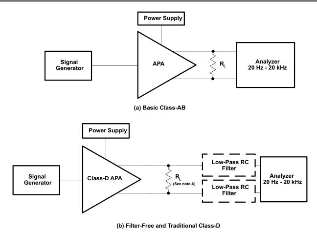
A. For efficiency measurements with filter-free Class-D, R<sub>1</sub> should be an inductive load like a speaker.
