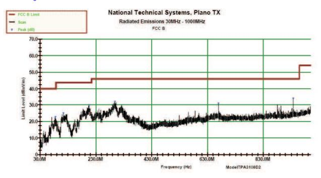
Figure 28. Radiated Emissions Prescan 30 MHz - 1000 MHz
