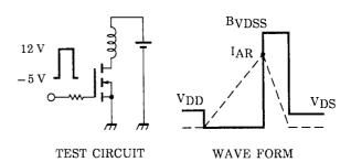
$$\begin{array}{l} T_{ch} = 25^{\circ}\text{C (Initial)} \\ \text{Peak I}_{AR} = 5 \text{ A}, \text{ R}_{G} = 25 \, \Omega \\ \text{V}_{DD} = 16 \text{ V}, \text{ L} = 1.0 \text{ mH} \end{array} \\ \text{EAS} = \frac{1}{2} \cdot \text{L} \cdot \text{I}^{2} \cdot (\frac{\text{BVDSS}}{\text{BVDSS} - \text{V}_{DD}})$$
