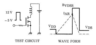
$$\begin{array}{l} T_{ch} = 25^{\circ} C \ (Initial) \\ Peak \ I_{AR} = 5 \ A, \ R_G = 25 \ \Omega \\ V_{DD} = 16 \ V, \ L = 1.0 \ mH \end{array} \\ \begin{array}{l} E_{AS} = \frac{1}{2} \cdot L \cdot I^2 \cdot ( \ \frac{B_{VDSS}}{B_{VDSS} - V_{DD}}) \end{array}$$
