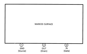
Note: That because of its MOS structure, this product is sensitive to static electricity.
