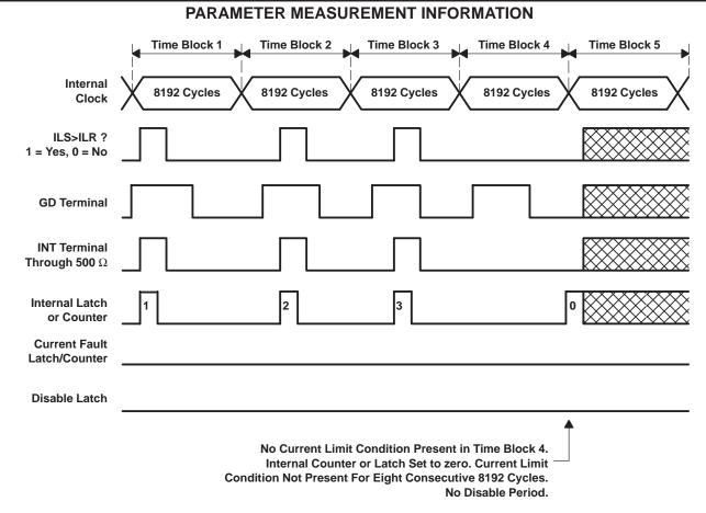
Figure 6. Current Fault Timing Diagram, Normal State
