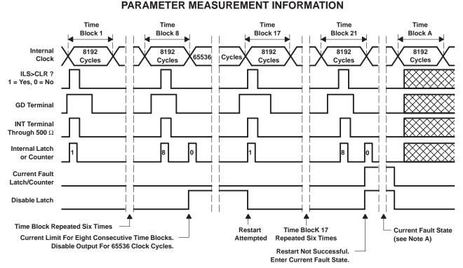
NOTE A: The integrated circuit remains in this state until cycled through the sleep state into the run state. Timing resumes as shown in time block A at right.
