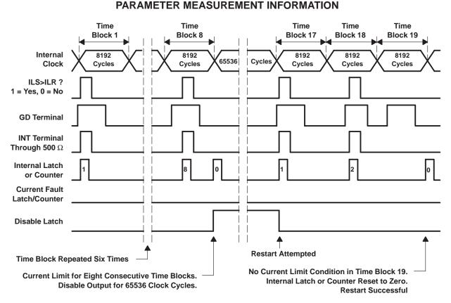
Figure 7. Current Fault Timing Diagram, Over-Current Limit Condition
