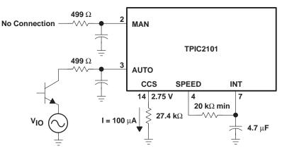
Figure 2. Automatic Mode Connections
