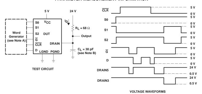
**Figure 1. Typical Operation Mode**
