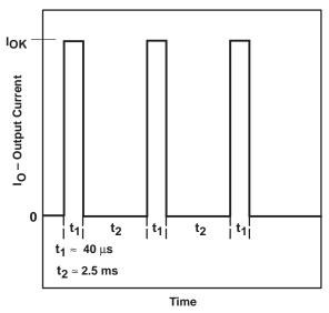
First output current pulses after turn-on in chopping mode with resistive load.
