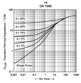
The single-pulse curve represents measured data. The curves for various pulse durations are based on the following equation:
