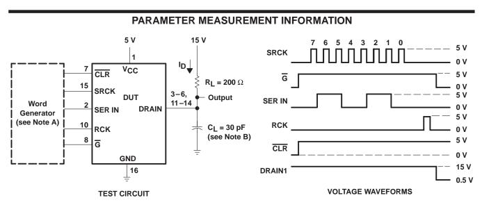
NOTES: A. The word generator has the following characteristics:  $t_{\Gamma} \le 10$  ns,  $t_{W} = 300$  ns, pulsed repetition rate (PRR) = 5 kHz,  $Z_{O} = 50~\Omega$ .
