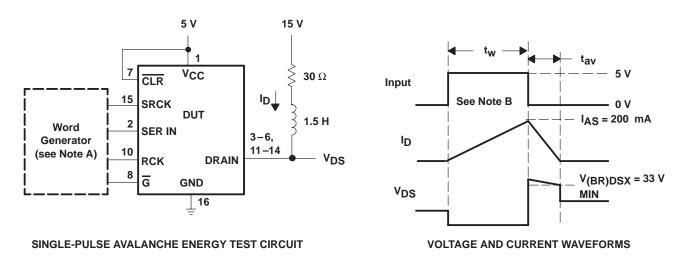
NOTES: A. The word generator has the following characteristics:  $t_r \le 10$  ns,  $t_f \le 10$  ns,  $Z_O = 50 \Omega$ .
