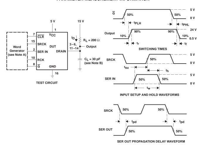
NOTES: A. The word generator has the following characteristics:  $t_{\Gamma} \le 10$  ns,  $t_{W} = 300$  ns, pulsed repetition rate (PRR) = 5 kHz,  $Z_{Q} = 50 \ \Omega$ .
