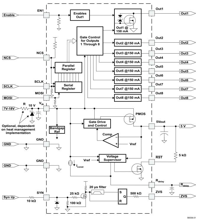
The value R is chosen based on maximum 5-V out load and minimum operating voltage desired. The Zener on the  $V_{IN}$  line helps limit the excess power dissipation within the IC when the operating voltage exceeds 10 V (starts conducting). For 12-V to 7-V operating input, the resistor and Zener are NOT required.
