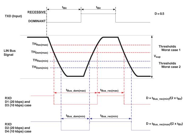
Figure 5. Definition of Bus Timing Parameters
