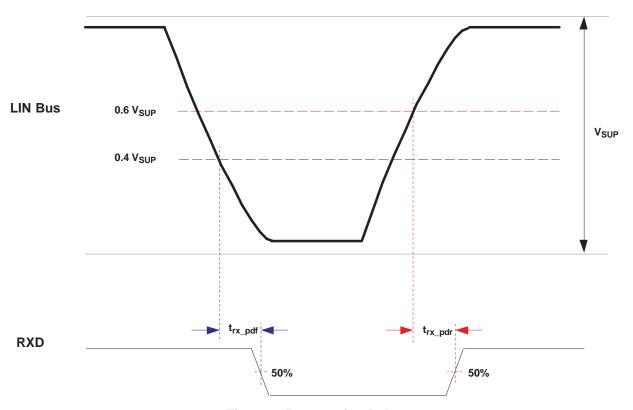
Figure 6. Propagation Delay
