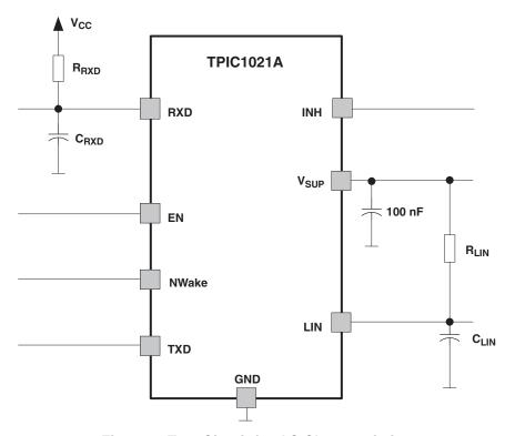
Figure 7. Test Circuit for AC Characteristics
