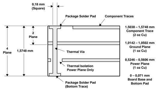
Figure 8. Multilayer Board (Side View)
