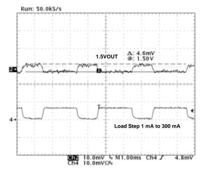
NOTE: Load regulation on 1.5VOUT with a load step of 1 mA to 300 mA.
