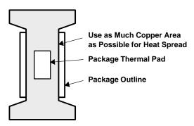
Figure 9. Land Configuration for Single-Layer PCB
