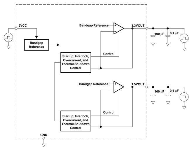
NOTE: The  $100-\mu$ F capacitor has: ESL = 3 nH and ESR =  $0.5 \Omega$  to  $1 \Omega$ . Testing circuit includes  $100-\mu$ F aluminum capacitors which may be replaced with  $10-\mu$ F ceramic capacitors. Both capacitors must have equivalent series inductance ESL < 3 nH and equivalent series resistance ESR <  $1 \Omega$ .
