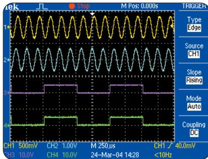
▶ *Four IsolatedChannel™ inputs and isolated external trigger input for quick, accurate, affordable floating and differential measurements.*
