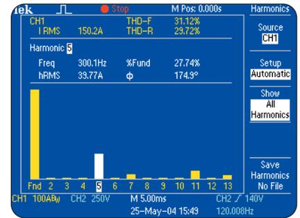
▶ *Conduct harmonic distortion measurements with TPS2PWR1 software.*
