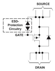
NOTE A: For all applications, all source terminals should be connected and all drain terminals should be connected.
