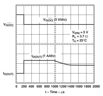
Figure 15. 3.7- $\Omega$  Load Connected to an Enabled TPS2021 Device
