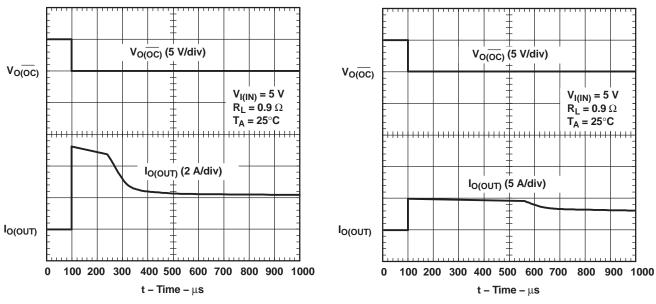
Figure 20. 0.9- $\Omega$  Load Connected to an Enabled TPS2023 Device
