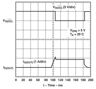
Figure 8. TPS2021, Ramped Load on Enabled Device
