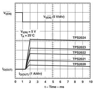
Figure 6. Device Enabled Into Short
