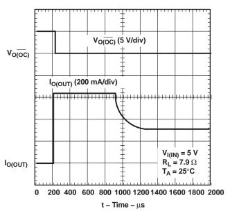
Figure 13. 7.9- $\Omega$  Load Connected to an Enabled TPS2020 Device
