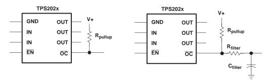
Figure 39. Typical Circuit for OC Pin and RC Filter for Damping Inrush OC Responses
