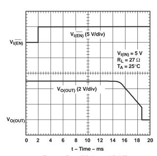
Figure 3. Turnoff Delay and Fall Time
