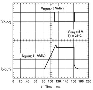
Figure 10. TPS2023, Ramped Load on Enabled Device
