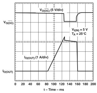
Figure 11. TPS2024, Ramped Load on Enabled Device
