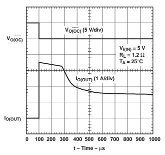
Figure 18. 1.2-Ω Load Connected to an Enabled TPS2022 Device
