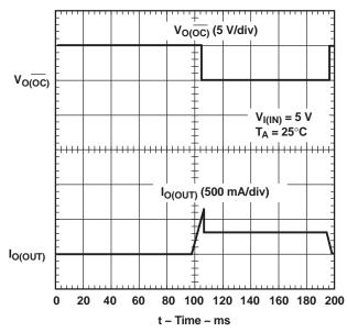
Figure 7. TPS2020, Ramped Load on Enabled Device
