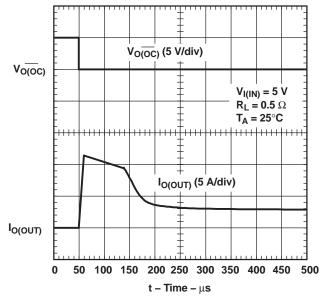
Figure 22. 0.5-Ω Load Connected to an Enabled TPS2024
