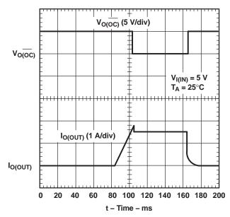
Figure 9. TPS2022, Ramped Load on Enabled Device
