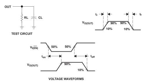
Figure 1. Test Circuit and Voltage Waveforms
