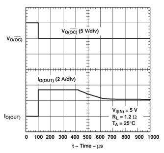
Figure 19. 1.2-Ω Load Connected to an Enabled TPS2023
