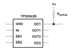
Figure 29. Typical Circuit for the OC Pin (Example, TPS2042B)
