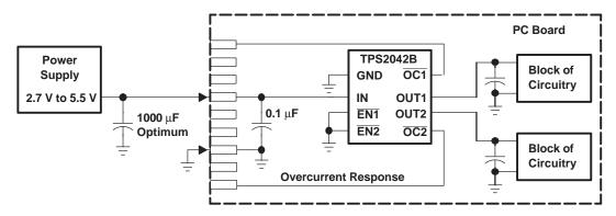
Figure 37. Typical Hot-Plug Implementation (Example, TPS2042B)
