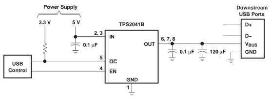
Figure 30. Typical One-Port USB Host / Self-Powered Hub
