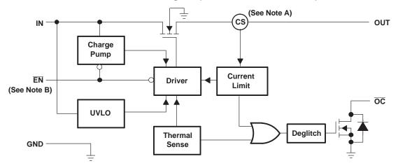
Note A: Current sense Note B: Active low (EN) for TPS2041B; Active high (EN) for TPS2051B
