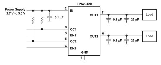
Figure 28. Typical Application (Example, TPS2042B)
