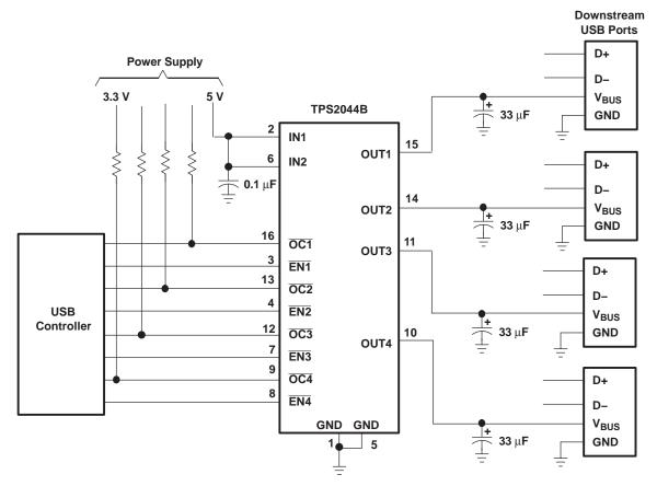
Figure 31. Typical Four-Port USB Host / Self-Powered Hub
