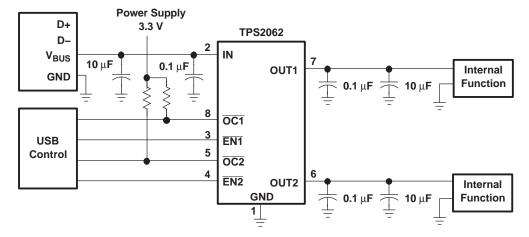
Figure 28. High-Power Bus-Powered Function
