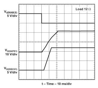
Figure 1. Turnon Voltage Transition of Channel 1
