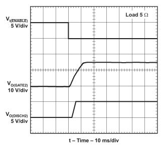
Figure 3. Turnon Voltage Transitioin of Channel 2
