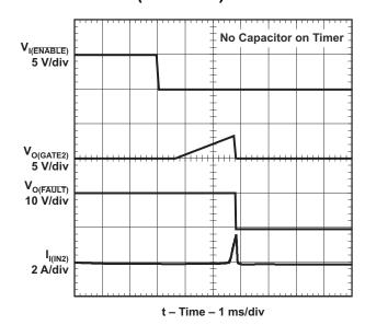
Figure 10. Channel 1 - Enabled Into Short Circuit
