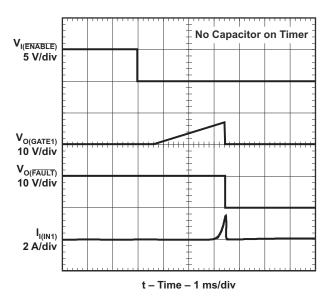
Figure 9. Channel 1 - Enabled Into Short Circuit
