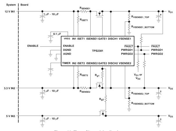
Figure 28. Three-Channel Application
