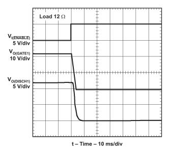
Figure 2. Turnoff Voltage Transition of Channel 1
