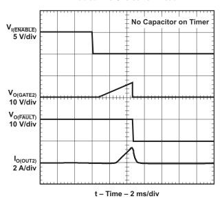
Figure 7. Channel 2 Overcurrent Response: Enabled Into Overcurrent Load
