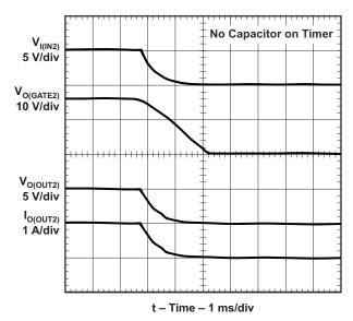
Figure 14. Channel 2 - Hot Removal
