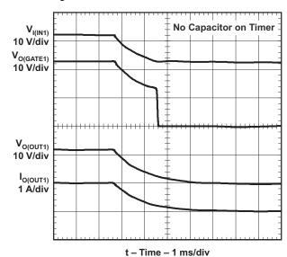
Figure 12. Channel 1 - Hot Removal
