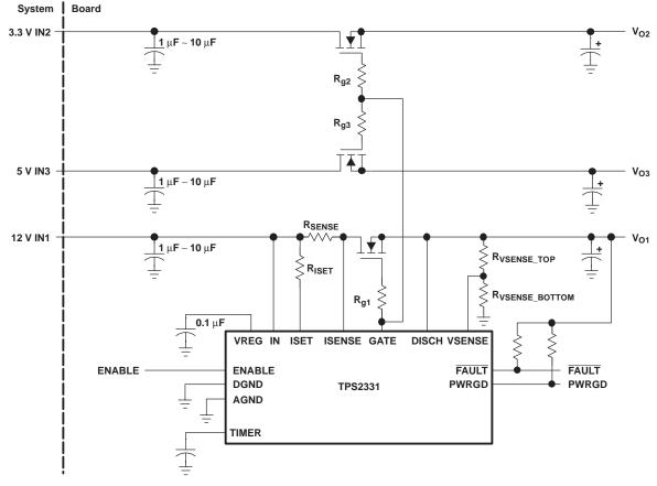
Figure 19. Three-Channel Application
