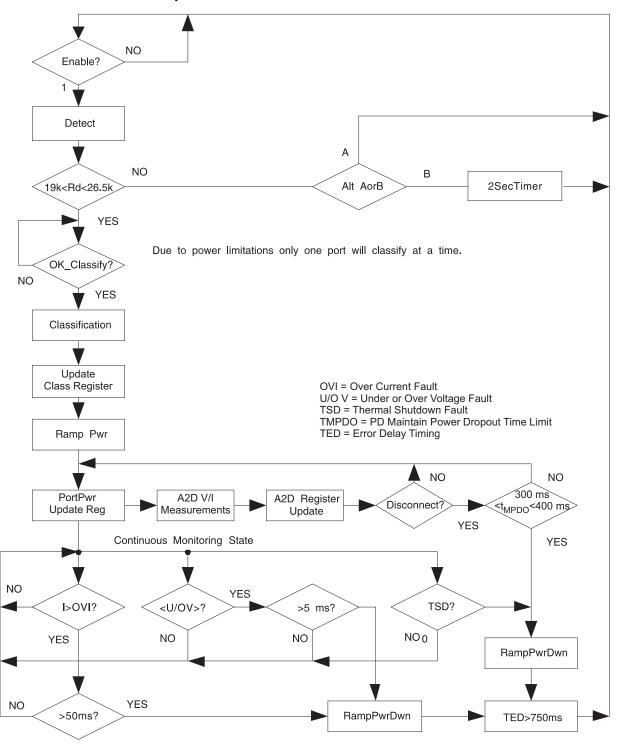
Figure 1. The Basic Flow for Auto Mode
