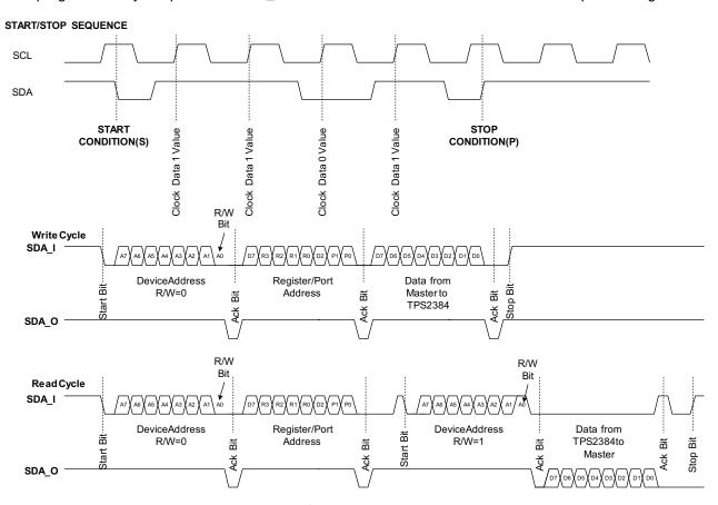
Figure 16. I<sup>2</sup>C Read/Write Cycles
