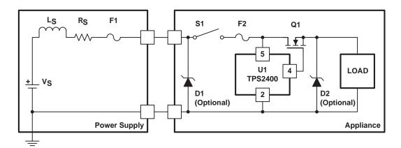
Figure 3. TPS2400 Application Block Diagram
