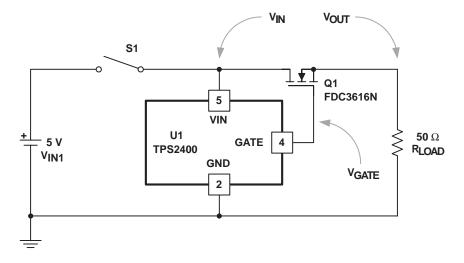
Figure 7. Output Turn-On Response Test Circuit
