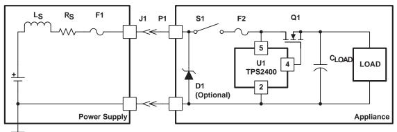
Figure 5. Turn-On Voltage Slew Rate Control Using the TPS2400
