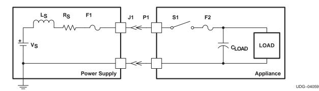
Figure 4. Power-Supply Output Resistance and Inductance Circuit Model
