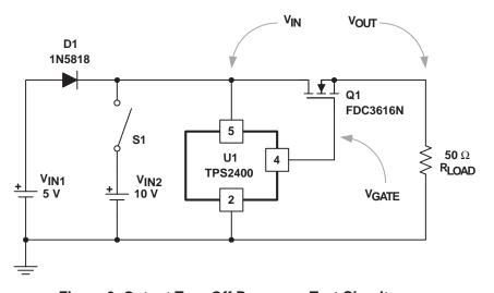
Figure 9. Output Turn-Off Response Test Circuit
