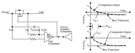
Figure 14. Fast Comparator Input Filtering
