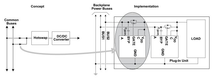
Figure 13. Example ORing of Input Power Buses
