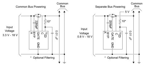
Figure 16. V<sub>DD</sub> Powering Examples
