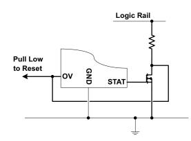
Figure 17. Use of STAT and OV to Latch TPS2411 OFF
