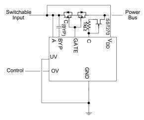
Figure 18. Bidirectional Blocking Example
