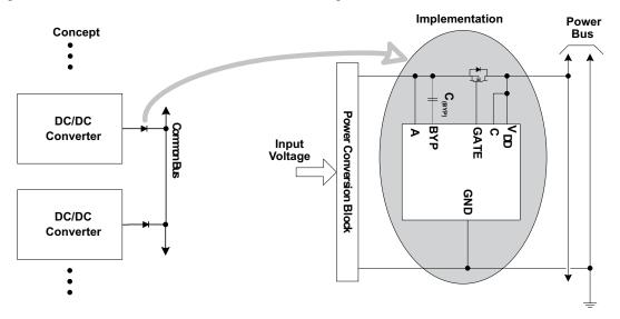
Figure 12. N+1 Power Supply Example
