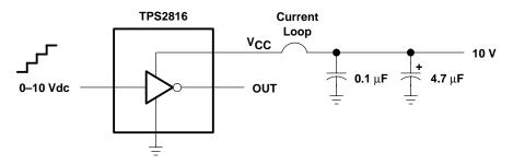
Figure 3. Shoot-Through Current Test Setup
