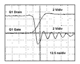
Figure 25. Q1 Turn-Off Waveform
