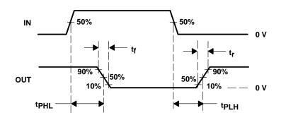
Figure 1. Typical Timing Diagram (TPS2816)
