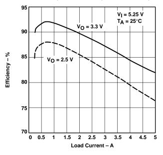
Figure 26. Converter Efficiency
