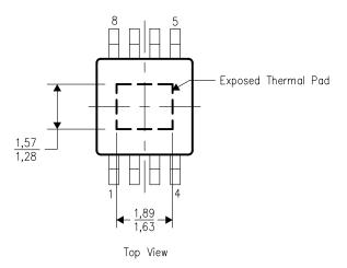
NOTE: All linear dimensions are in millimeters
