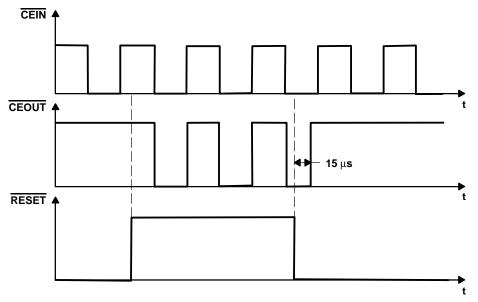
Figure 2. Chip-Enable Timing
