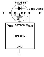
Figure 3. Driving an External MOSFET Transistor With BATTON
