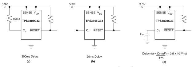
Figure 14. Configuration Used to Set the RESET Delay Time
