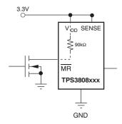
Figure 13. Using an External MOSFET to Minimize I<sub>DD</sub> When MR Signal Does Not Go to V<sub>DD</sub>
