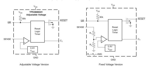
Figure 1. Adjustable and Fixed Voltage Versions
