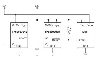
Figure 12. Using MR to Monitor Multiple System Voltages
