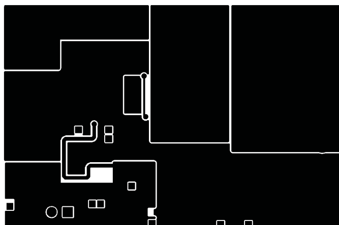
Figure 46. TPS40200EVM-001 Bottom Copper (X-Ray View from Top)
