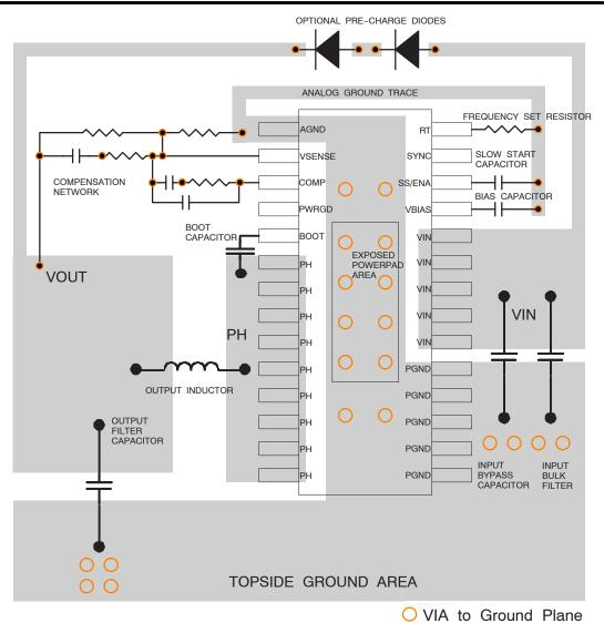
Figure 10. TPS54973 PCB Layout
