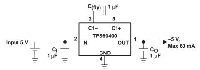
Figure 23. Typical Operating Circuit
