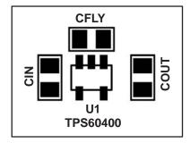
Figure 37. Recommended PCB Layout for TPS6040x (top layer)
