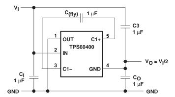
Figure 26. TPS60400 as a High-Efficiency Rail Splitter
