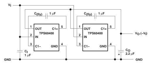
Figure 29. Paralleling Devices
