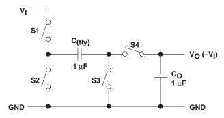
Figure 1. Operating Principle
