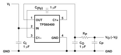
Figure 24. TPS60400 and TPS60401 With RC-Post Filter
