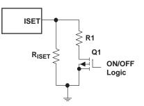
Figure 13. Switching In/Out an Additional Resistor to Change Output Current
