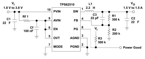
Figure 24. Adjustable Version Programmed to 1.5 V Using Power Good
