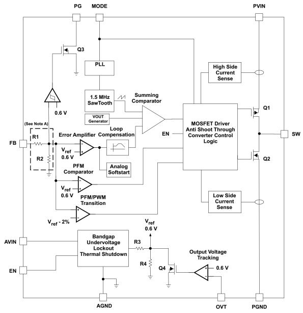
A. R1 and R2 are only used for the fixed output voltage version.
