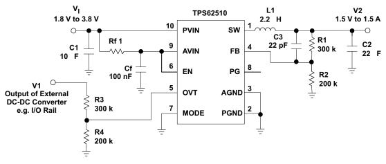
Figure 18. Output Voltage Tracking, V2 Tracks V1
