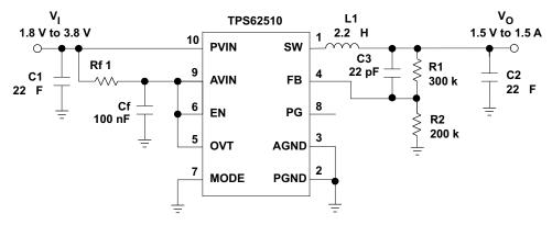
Figure 23. Adjustable Version Programmed to 1.5 V
