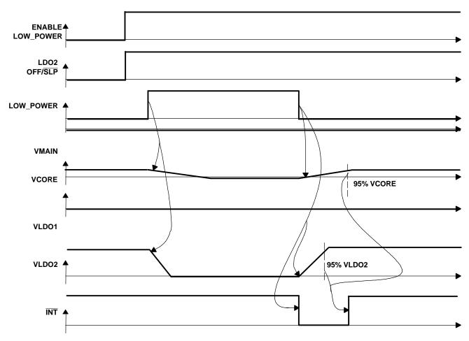
Figure 33. State 2 to State 3 Transition. VCORE Lowered, LDO2 Disabled. Subsequent State 3 to State 2 Transition When LOW POWER Is De-asserted.
