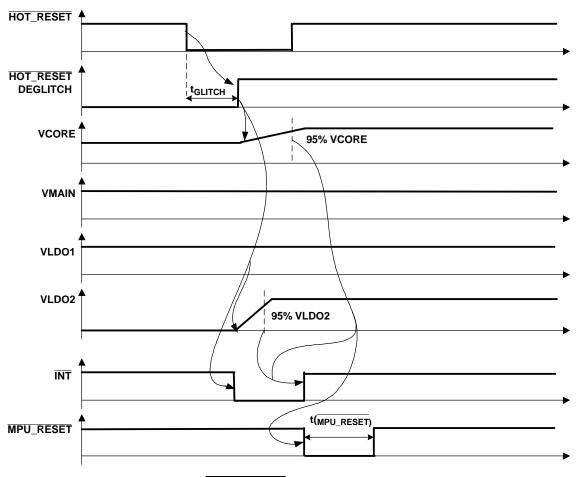
Figure 35. State 3 to State 2 Transition (HOT\_RESET Activated, See Interrupt Management Section for INT Behavior)
