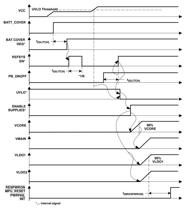
Figure 31. State 1 to State 4 to State 2 Transition (Power-up behavior when V<sub>CC</sub> ramp is longer than 2.4 ms)
