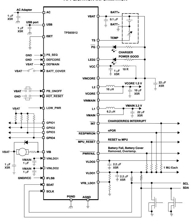
Figure 43. Typical Application Circuit
