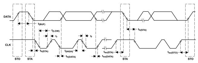
Figure 42. Serial Interface Timing Diagram
