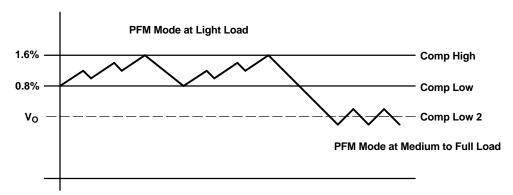
Figure 28. Power-Save Mode Thresholds and Dynamic Voltage Positioning
