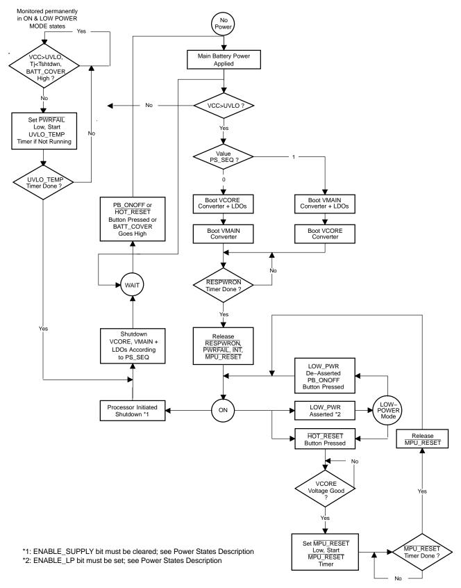
Figure 29. TPS65012 Power-On State Diagram
