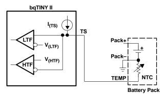
Figure 26. TS Pin Configuration
