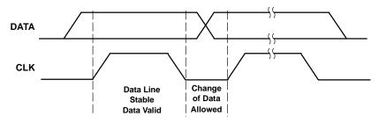
Figure 37. Bit Transfer on the Serial Interface
