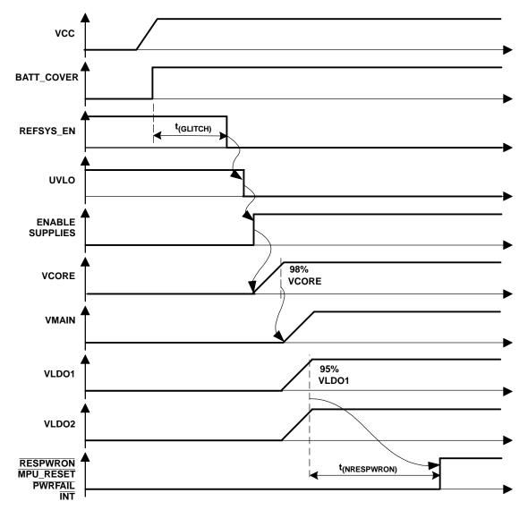
Figure 30. State 1 to State 2 Transition (PS\_SEQ=0,  $V_{CC} > V_{UVLO} + HYST$ )
