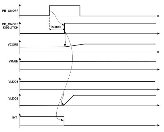
Figure 34. State 3 to State 2 Transition. PB\_ONFF Activated (See Interrupt Management Section for INT Behavior)
