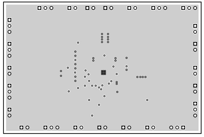
Figure 3. Layer 2, GND Plane
