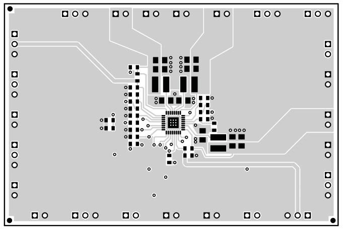
Figure 2. Top Layer Routing
