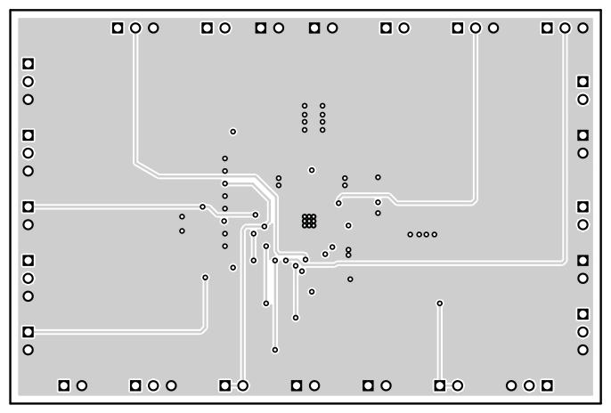
Figure 5. Bottom Layer Routing
