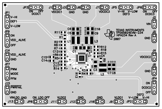
Figure 1. Assembly Layer
