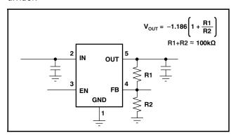
Figure 27. TPS72301 Adjustable LDO Regulator Programming
