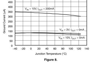
**GROUND CURRENT vs JUNCTION TEMPERATURE**
