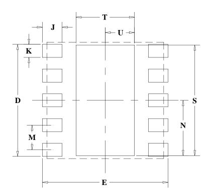
Recommended PC board layout to Accept 10 Pin Module Package:
