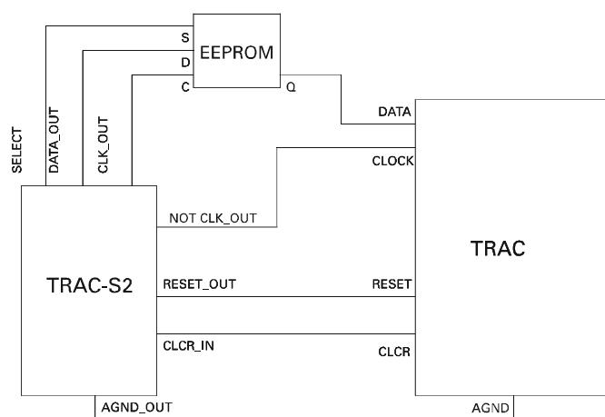
Connections between the support circuit, the EEPROM and the TRAC device are shown above.
