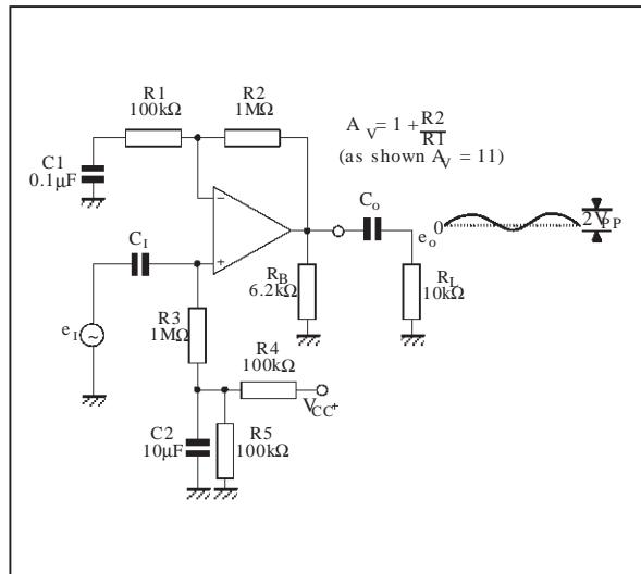
**NON-INVERTING DC GAIN**
