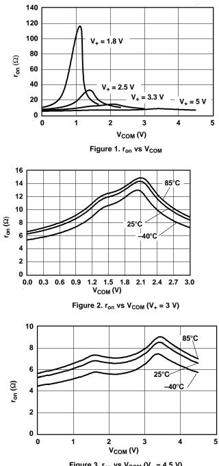
Figure 3.  $r_{on}$  vs V<sub>COM</sub> (V<sub>+</sub> = 4.5 V)
