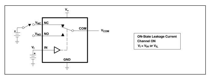
Figure 15. ON-State Leakage Current (I<sub>COM(ON)</sub>, I<sub>NC(ON)</sub>, I<sub>NO(ON)</sub>)
