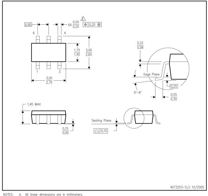
A. All linear dimensions are in millimeters.
