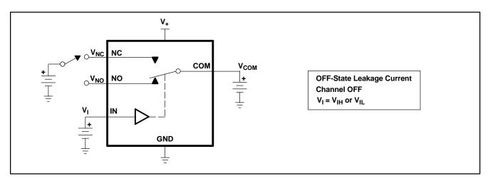
Figure 14. OFF-State Leakage Current (I<sub>NC(OFF)</sub>, I<sub>NO(OFF)</sub>)
