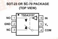
The TS5A3157 is a single-pole double-throw (SPDT) analog switch that is designed to operate from 1.65 V to 5.5 V. This device can handle both digital and analog signals, and signals up to  $V_+$  can be transmitted in either direction.
