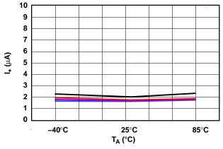
Figure 12. Power-Supply Current vs Temperature  $(V_{+} = 5 V)$
