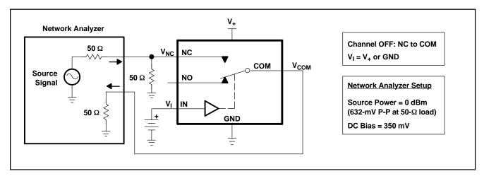
Figure 20. OFF Isolation (O<sub>ISO</sub>)
