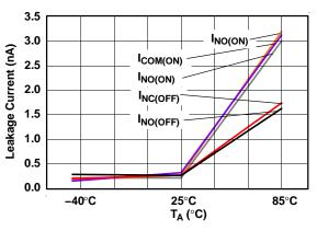
Figure 4. Leakage Current vs Temperature (V<sub>+</sub> = 5.5 V)
