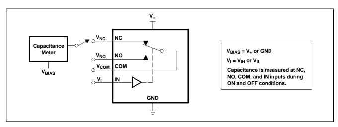
Figure 16. Capacitance (C<sub>1</sub>, C<sub>COM(ON)</sub>, C<sub>NC(OFF)</sub>, C<sub>NO(OFF)</sub>, C<sub>NC(ON)</sub>, C<sub>NO(ON)</sub>)
