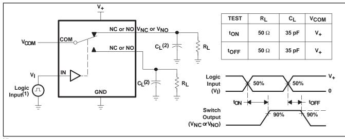
(1) All input pulses are supplied by generators having the following characteristics: PRR  $\leq$  10 MHz, Z<sub>O</sub> = 50  $\Omega$ , t<sub>f</sub> < 5 ns, t<sub>f</sub> < 5 ns. (2) C<sub>1</sub> includes probe and jig capacitance.
