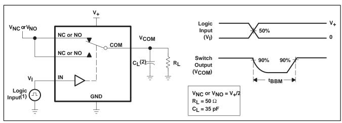
(1) All input pulses are supplied by generators having the following characteristics: PRR  $\leq$  10 MHz, Z<sub>O</sub> = 50  $\Omega$ , t<sub>f</sub> < 5 ns, t<sub>f</sub> < 5 ns. (2) C<sub>1</sub> includes probe and jig capacitance.
