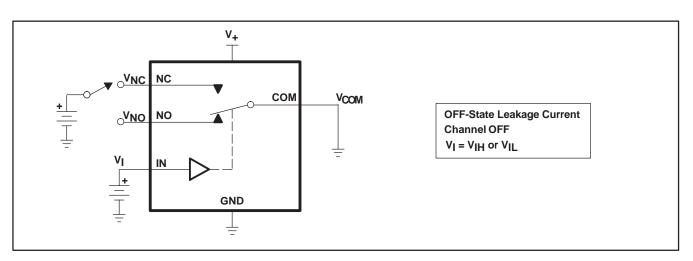
Figure 12. OFF-State Leakage Current (I<sub>NC(OFF)</sub>, I<sub>NO(OFF)</sub>)
