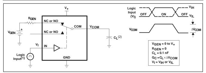
(1) All input pulses are supplied by generators having the following characteristics: PRR  $\leq$  10 MHz, Z<sub>O</sub> = 50  $\Omega$ , t<sub>f</sub> < 5 ns, t<sub>f</sub> < 5 ns. (2) C<sub>L</sub> includes probe and jig capacitance.
