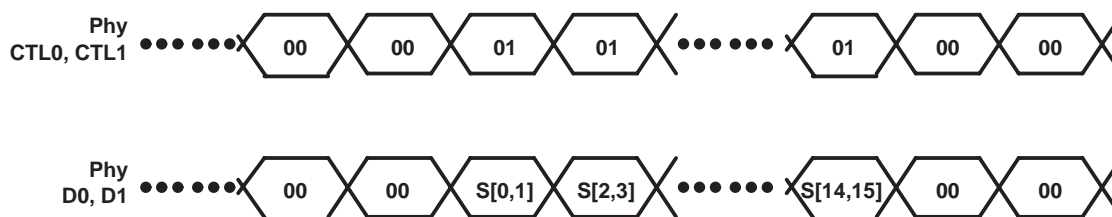
Figure 5. Status Transfer Timing
