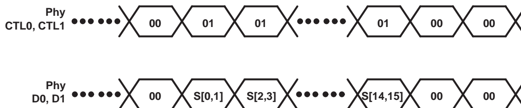
Figure 12. Status Transfer Timing
