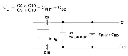
Figure 8-4. Load Capacitance for the TSB43AA22 PHY
