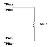
Figure 9-1. Test Load Diagram
