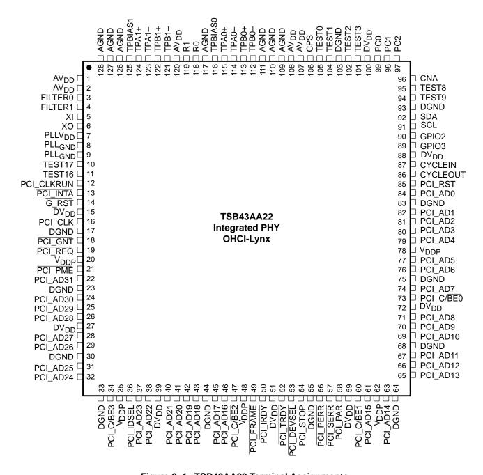
Figure 2–1. TSB43AA22 Terminal Assignments
