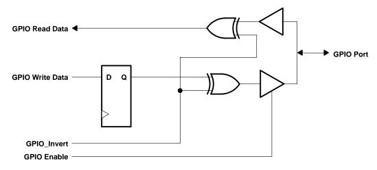
Figure 7–1. GPIO2 and GPIO3 Logic Diagram
