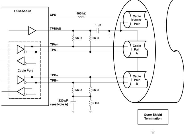
NOTE A: The IEEE 1394-1995 standard calls for a 250-pF capacitor, which is a nonstandard component value. A 220-pF capacitor is recommended.
